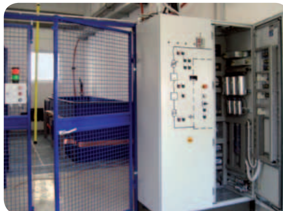
Lastwechselpfahrungen an MS-Kabelgarnituren Load-cycle tests on MV cable accessories
